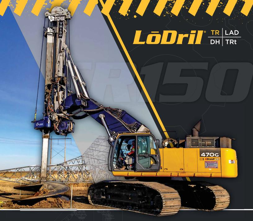
**TR150** Our TR150 boasts 150,000 ft-lbs of torque and 35,000 ft-lbs of crowd force, making it a foundation drilling powerhouse. Key features include a 40,000 ft-lbs (max line pull) Kelly winch, compatibility with augers ranging from 18 inches to 14 feet in diameter, an impressive range of drilling depth from 30 to 100 feet, a crowd stroke of 168 to 228 inches per pass (depending on configuration), and improved transportability with the option to disconnect the attachment from the carrier.
