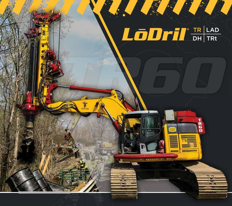
Boasting 66,000 ft-lbs of rotary torque, a maximum hole depth of 80 feet, and equipped with a fully integrated Kelly winch, the powerful TR60 is a crucial member of our TR Series. As customizable as it is efficient, this rig is available in a variety of mounting options, including truck, track, and excavator, giving you the freedom to decide how you want to drill.
