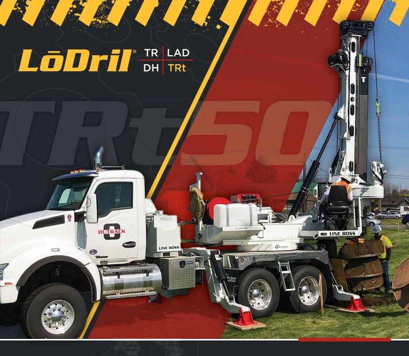
What would happen if the power and durability of a TR rig met the ease-of-use and maneuverability of a truck? That question was the genesis of our TRt series: truck-mounted rigs with easy-to-use controls and customized hydraulic solutions. A prominent member of the series, the TRt50 is impressive in its own right. Equipped with a high-capacity Kelly winch and capable of digging holes 48 inches wide and 80 feet deep, the TRt50 will take your productivity to the next level.
